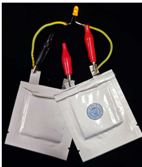
SI 33. pouch battery powering a small light bulb.
