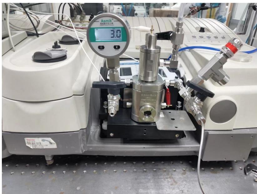
**Fig. S35.** Picture of the custom-made high-pressure spectroelectrochemical setup for SEIRAS investigation.
