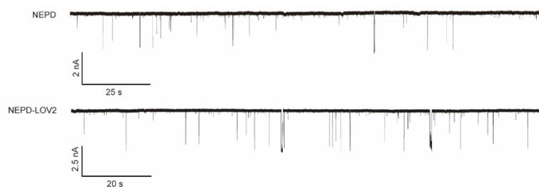
**Figure S3.** Additional raw current trace of NEPD and NEPD-LOV2 in figure 2a. All the data was acquired in 1 M KCl, 10 mM Tris-HCl, 1 mM EDTA, pH 7.40. All data is recorded with a sample rate of 100 kHz and filtered at 10 kHz.
