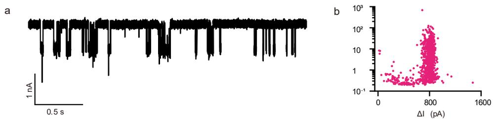
**Figure S5.** Supplemented data analysis of purified NEPD protein samples using 8.4nm-in-diameter solid-state nanopore. (a)The raw current trace of NEPD-LOV2 at 300mV voltage. (b) Scatter plots for duration vs  $\Delta I$  (right). Point: 272. All the data was acquired in 1 M KCl, 10 mM Tris-HCl, 1 mM EDTA, pH 7.40. All data is recorded with a sample rate of 100 kHz and filtered at 10 kHz.
