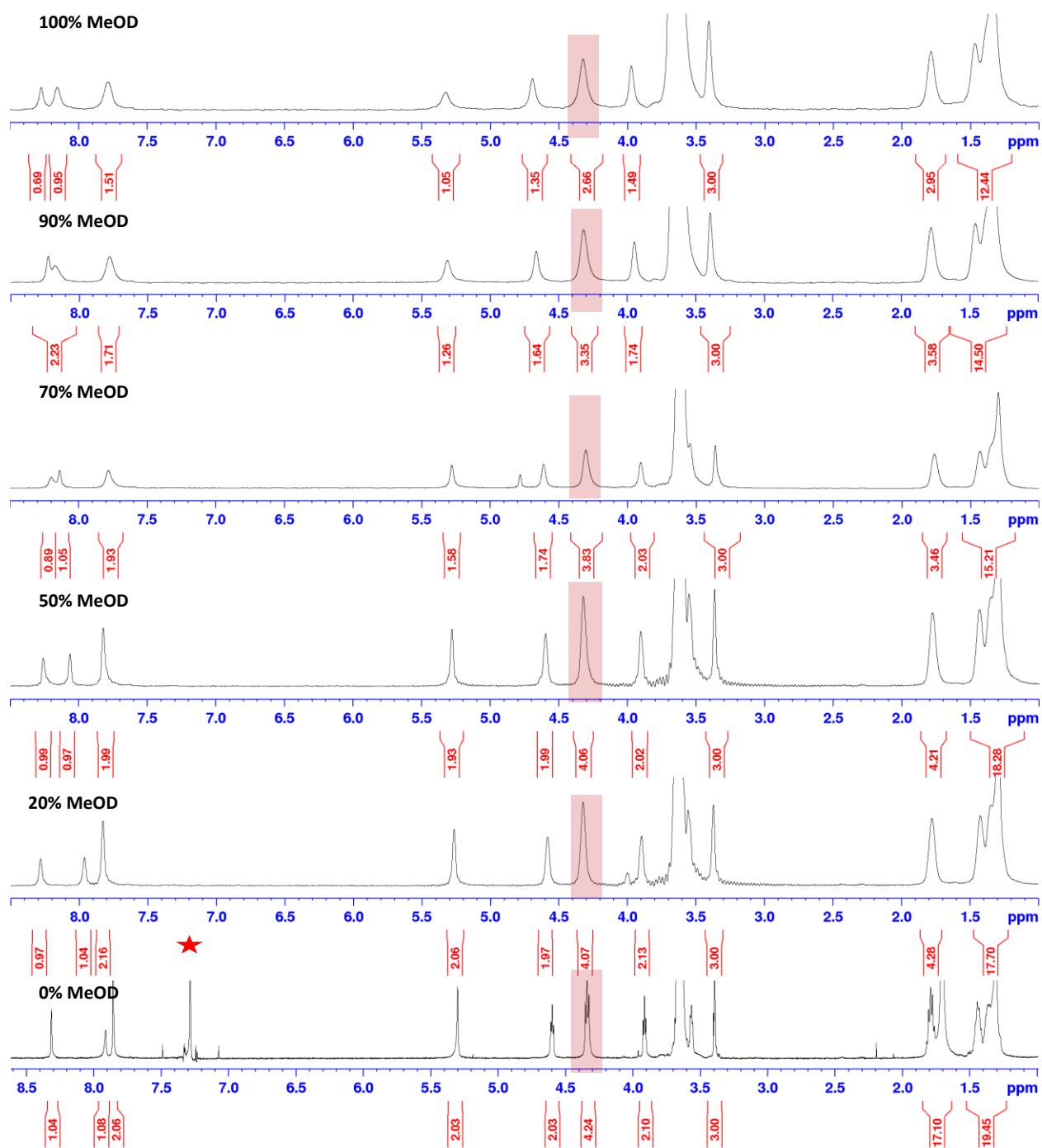
Figure S14: Stack plot of 1 H NMR spectra of PE 12 -g-PEG 750 in different CDCl 3 -MeOD compositions. Spectra where the solvent peaks are not visible (all, except 0 % MeOD) were recorded using the PFG self-diffusion sequence, which suppresses the solvent peaks. ★ represents the CHCl 3 peak in the spectra.
