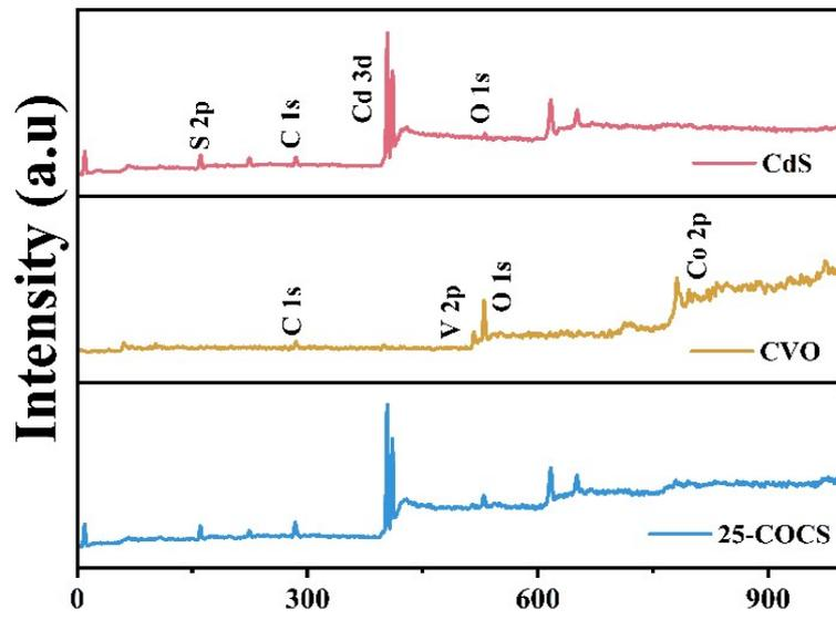
Fig. S3 XPS survey spectra for CdS, CVO and 25-COCS.
