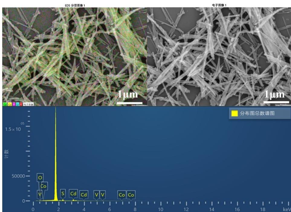
**Fig. S2** EDS layered images, electron images and element distribution spectra of 25-COCS.
