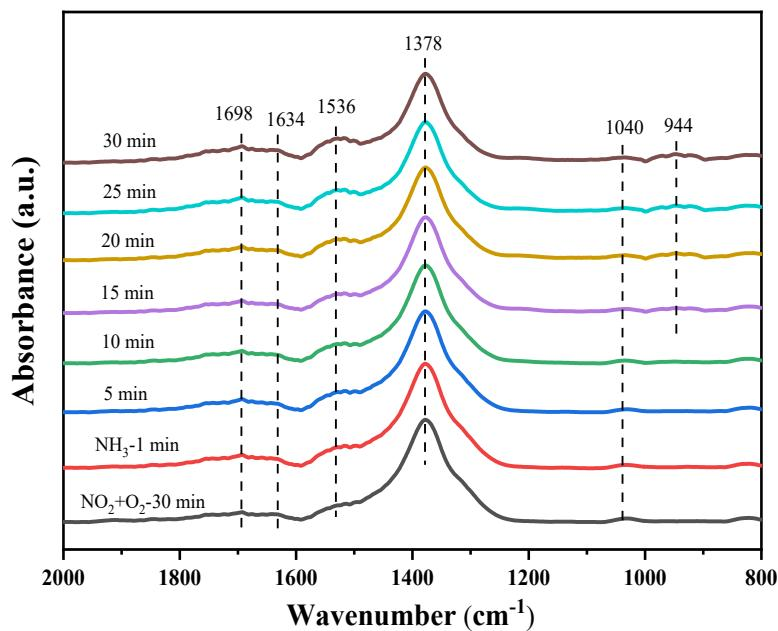
**Fig. S7.** In situ DRIFTS of  $\text{Mn}_3\text{Co}_2\text{NiO}_x$  catalysts with  $\text{NH}_3$  after pre-adsorption of  $\text{NO} + \text{O}_2$  for different times at 190°C
