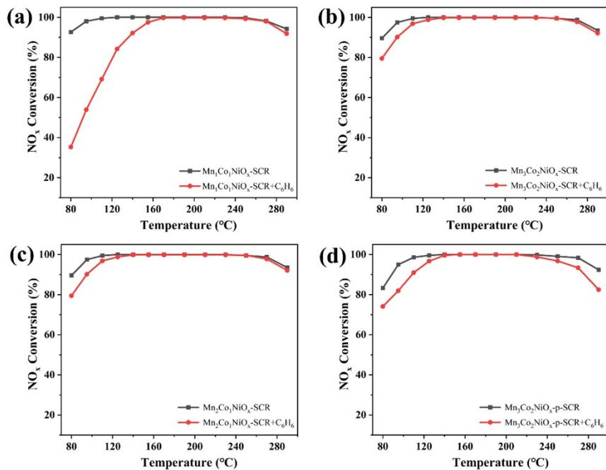
**Fig.S3.** (a) NO<sub>x</sub> conversion of catalysts with different manganese contents in different atmospheres (a) MnCo<sub>2</sub>NiO<sub>x</sub>; (b) Mn<sub>1</sub>Co<sub>1</sub>NiO<sub>x</sub>; (c) Mn<sub>3</sub>Co<sub>2</sub>NiO<sub>x</sub> ; (d) Mn<sub>3</sub>Co<sub>2</sub>NiO<sub>x</sub>-p
