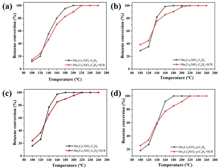
**Fig.S4.** (a) Benzene conversion of catalysts with different manganese contents in different atmospheres (a) MnCo<sub>2</sub>NiO<sub>x</sub>; (b) Mn<sub>1</sub>Co<sub>1</sub>NiO<sub>x</sub>; (c) Mn<sub>3</sub>Co<sub>2</sub>NiO<sub>x</sub> ; (d) Mn<sub>3</sub>Co<sub>2</sub>NiO<sub>x</sub>-p
