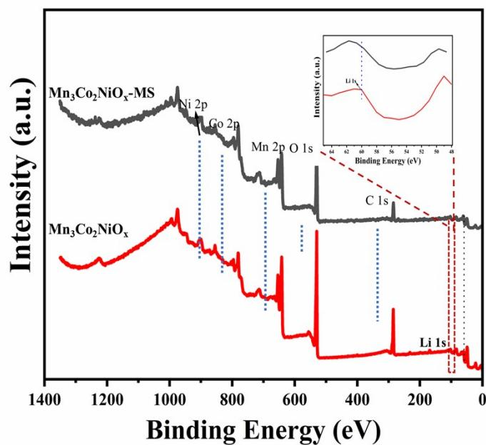
**Fig. S6** XPS survey spectra of  $\text{Mn}_3\text{Co}_2\text{NiO}_x$  and  $\text{Mn}_3\text{Co}_2\text{NiO}_x$ -MS
