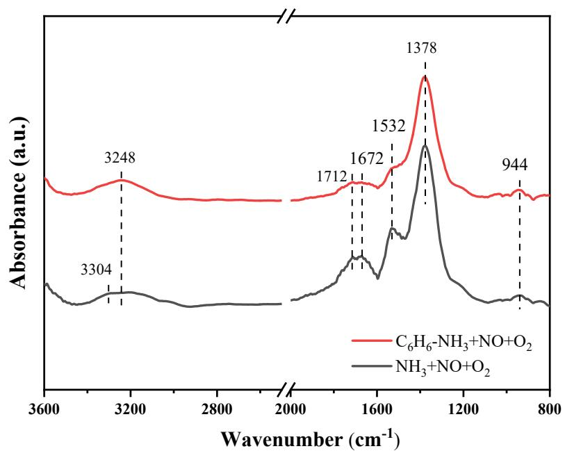
**Fig S8** In situ DRIFTS spectra of  $\text{Mn}_3\text{Co}_2\text{NiO}_x$  catalysts after reaction with SCR gases in the presence or absence of benzene at 190°C
