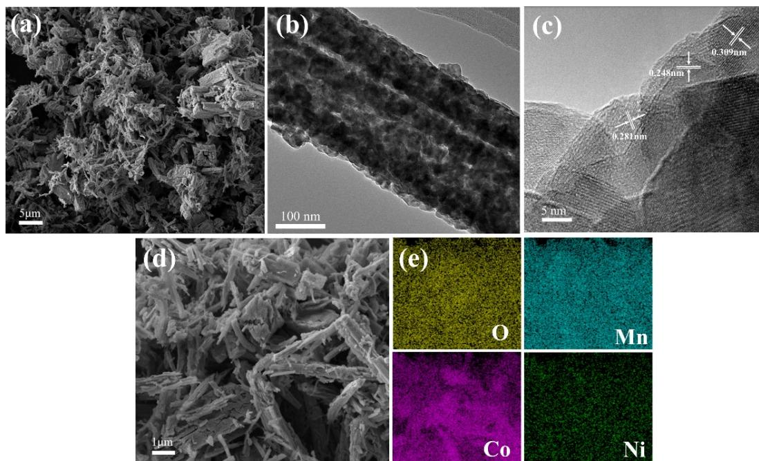
**Fig. S5** SEM images of  $\text{Mn}_3\text{Co}_2\text{NiO}_x\text{-MS}$  catalyst at (a) 5  $\mu\text{m}$  and (d) 1  $\mu\text{m}$ ; (b-c) HR-TEM images; (e-f) EDS elemental mapping of  $\text{Mn}_3\text{Co}_2\text{NiO}_x\text{-MS}$  catalyst
