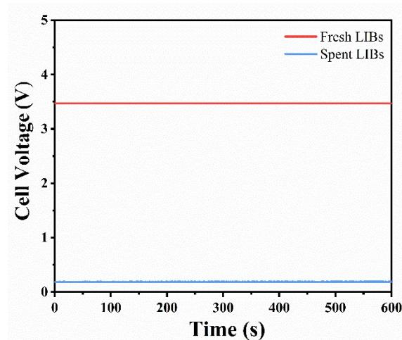
**Fig. S2** Open-circuit voltage of spent lithium-ion batteries after discharge
