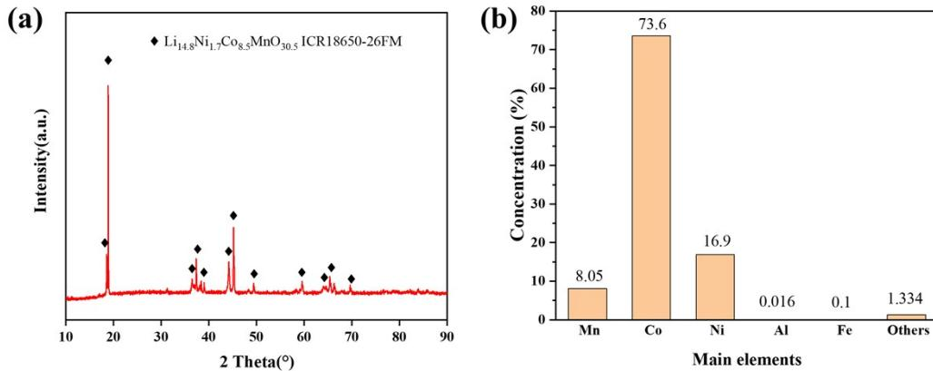
**Fig. S1** (a) XRD and (b) XRF images of spent LIBs.
