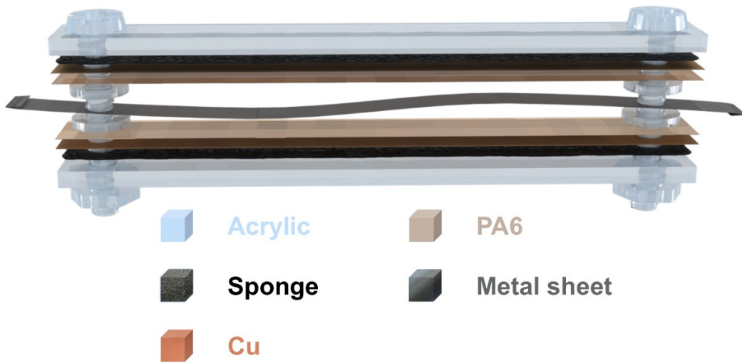
Fig. S3: Schematic of TENG with a metallic sheet as the vibration layer.
