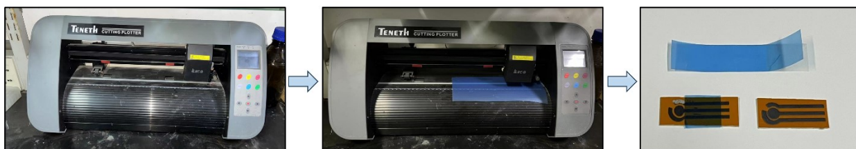
Fig. S1 The preparation to control reaction area of the integrated electrode.
