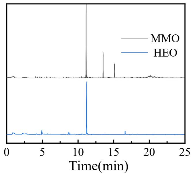
Figure S3. GC-MS spectra analysis of enriched tail gas after o-xylene oxidized by HEO and MMO.
