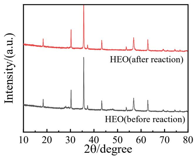
Figure S2. XRD patterns of the fresh HEO and spent HEO after reaction at 450 °C
