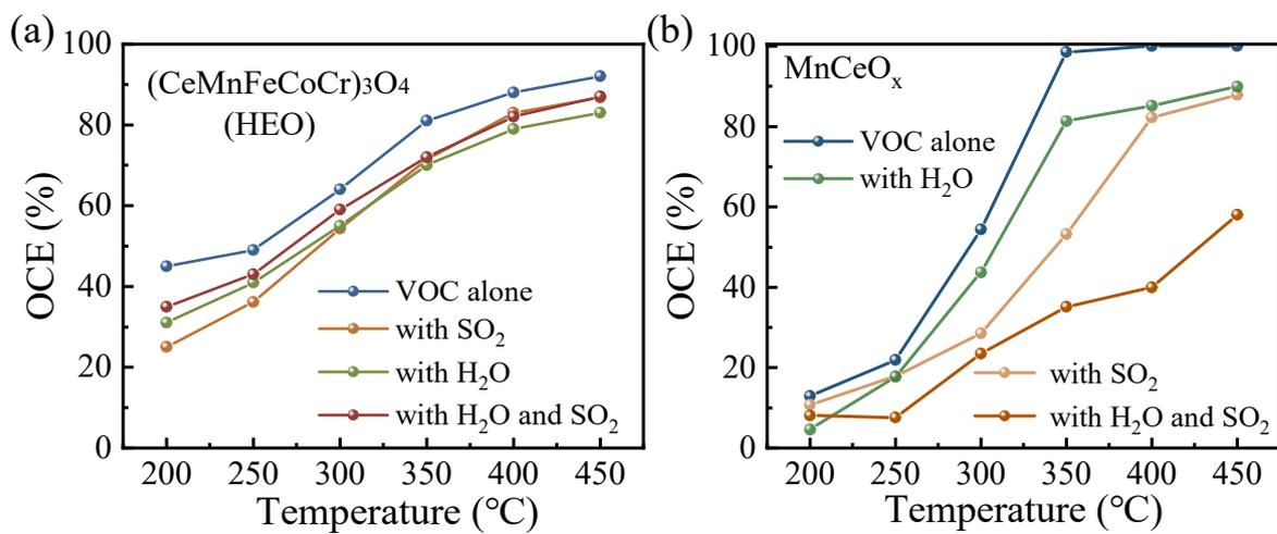
Figure S6. Comparison of catalytic oxidation activity between HEO (a) and conventional MnCeO<sub>x</sub> catalyst (b) for o-xylene degradation
