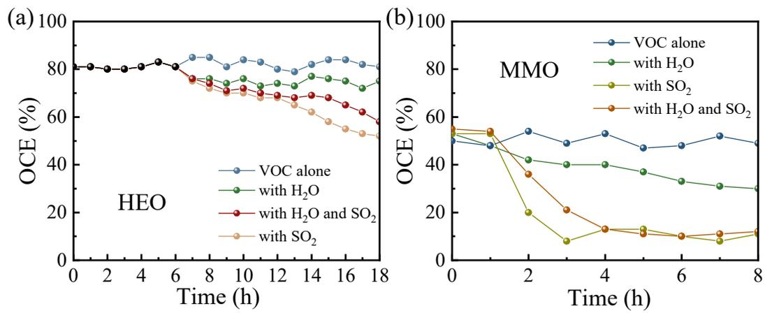
Fig. S7 Long-term stability of (a) HEO and (b) MnCeOx for o-xylene oxidation
