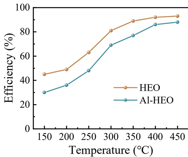
Figure S5. O-xylene removal efficiency of HEO and Al-HEO
