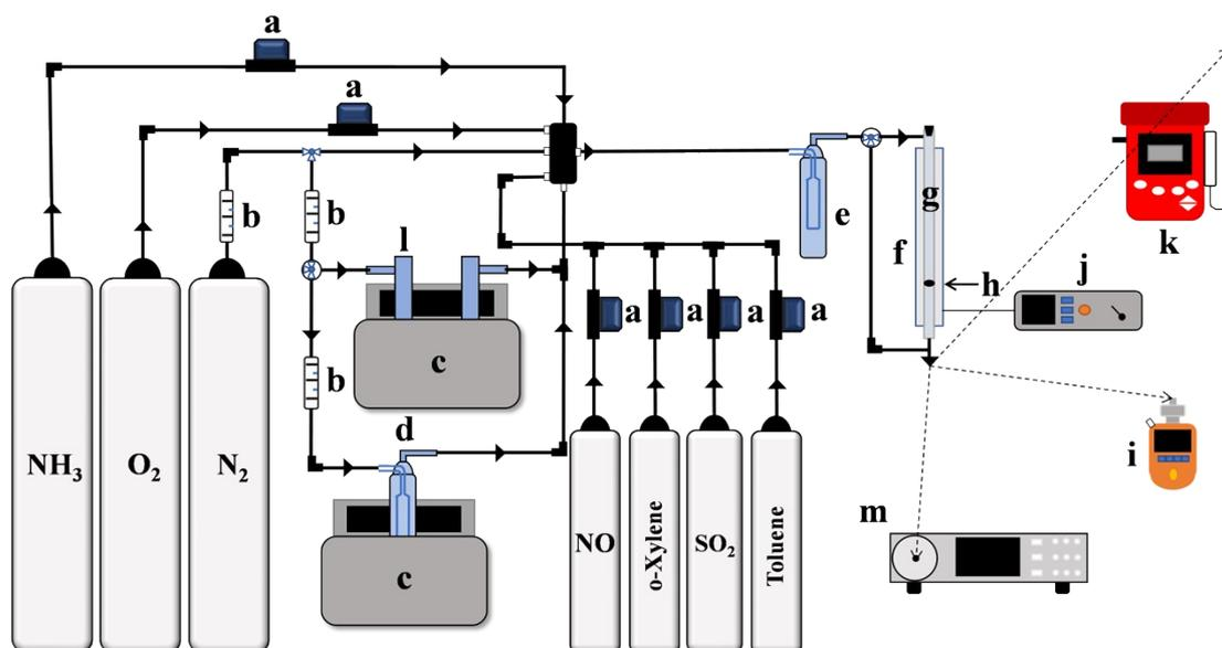
Figure S1. Schematic diagram of the experimental apparatus. Components (a: mass flow meter; b: volume flow meter; c: thermostatic bath; d: cleaning bottle for water vapor generation; e: cleaning bottle for gas mixing; f: heating device; g: quartz reactor; h: catalyst; i: gas detector; j: temperature controller; k: flue gas analyzer; l: Mercury generator; m: mercury analyzer)
