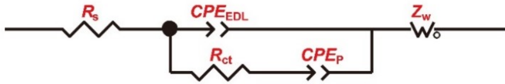
Fig. S14 The equivalent electric circuit model used for fitting the Nyquist plots. R_s : the intrinsic ohmic resistance; R_{ct} : charge transfer resistance; CPE_{EDL} : constant phase element representing the electrical double layer capacitance (EDLC); CPE_p : constant phase element representing the pseudocapacitance provided by the oxygen functional groups; Z_w : a Generalized Finite Warburg element terminating in an open circuit.
