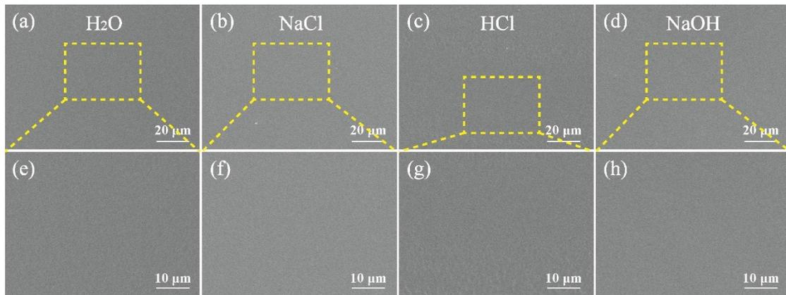
**Figure S7.** SEM image and enlarged SEM image of the fractured surface of pure TPU after 60 days of the chemical resistance test.
