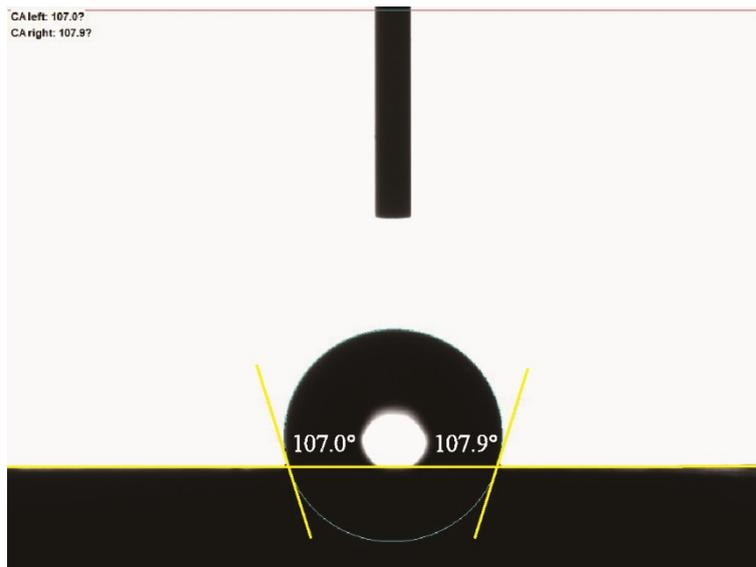
**Figure S3.** Water contact angles of TPU/ZIF-67.
