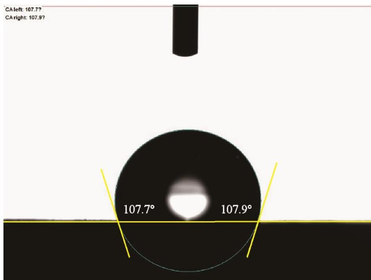
**Figure S6.** Water contact angles of TPU/h-BNNSs@Co.
