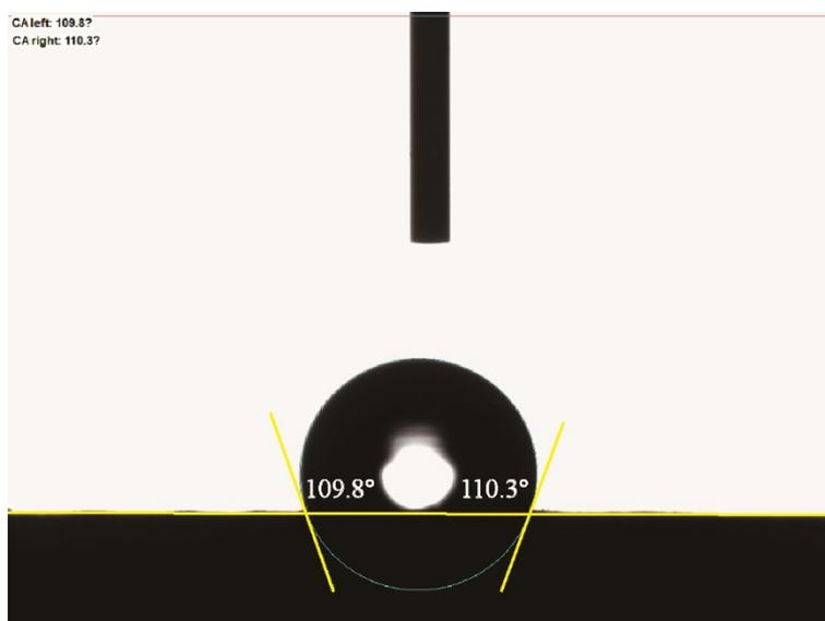
**Figure S2.** Water contact angles of pure TPU.
