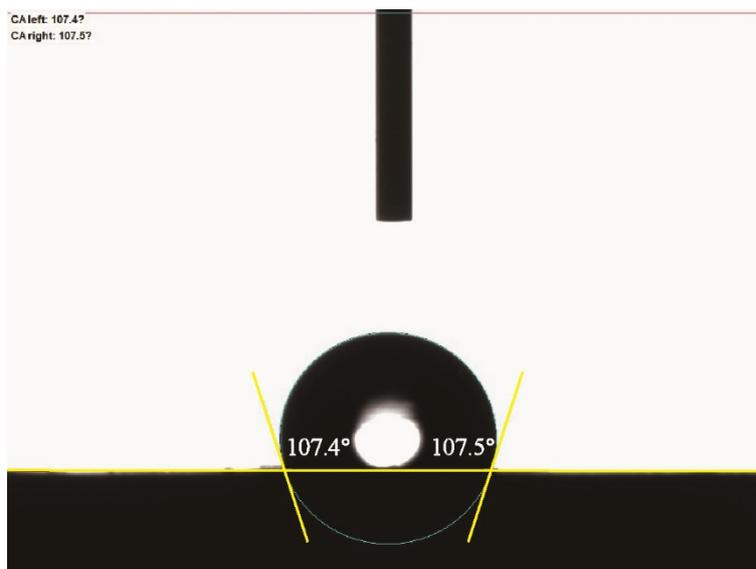
**Figure S4.** Water contact angles of TPU/NH<sub>2</sub>-ZIF-67.
