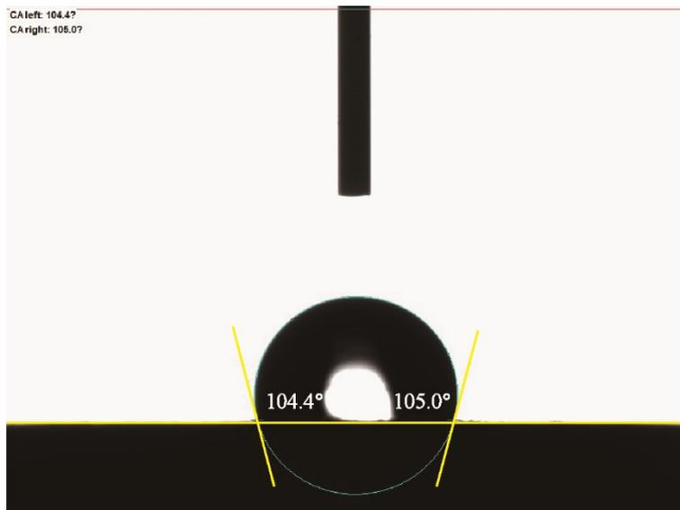
**Figure S5.** Water contact angles of TPU/BA@NH<sub>2</sub>-ZIF-67.
