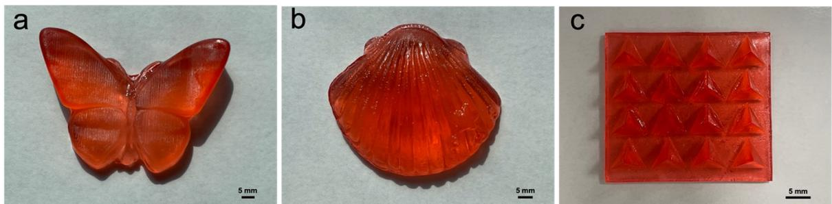
Figure S12. 3D printed items: a) butterfly, b) shell, and c) a square surface with pyramid structures.
