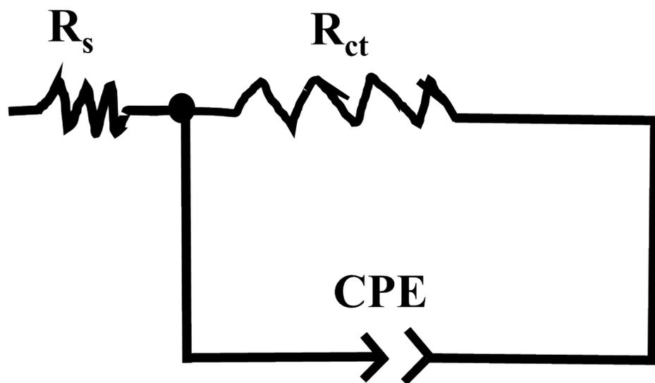
**Fig. S1** Equivalent circuit diagram for MD-Co/Ni-4 nanostructure.
