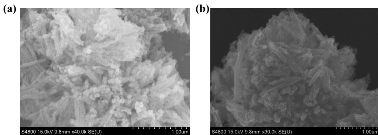
**Fig. S3** FESEM images: (a) prior to the cycling test and (b) post-cycling test.
