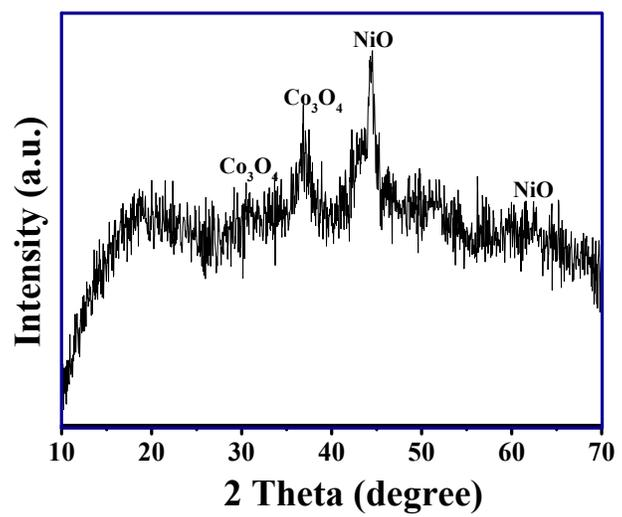
**Fig. S2** XRD pattern of the MD-Co/Ni-4 nanostructure post-cycling test.
