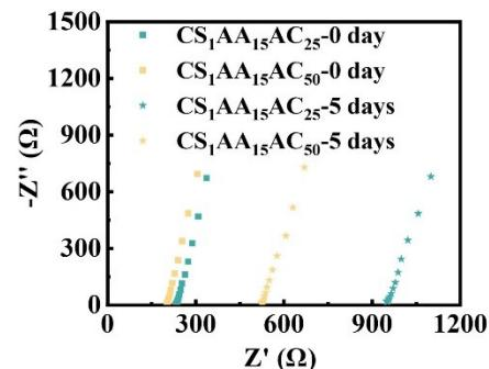
**Fig. S9:** Impedance of  $\text{CS}_1\text{AA}_{15}\text{AC}_{25}$ ,  $\text{CS}_1\text{AA}_{15}\text{AC}_{50}$  hydrogels initial and stored at 25 °C and 54% RH for 5 days.
