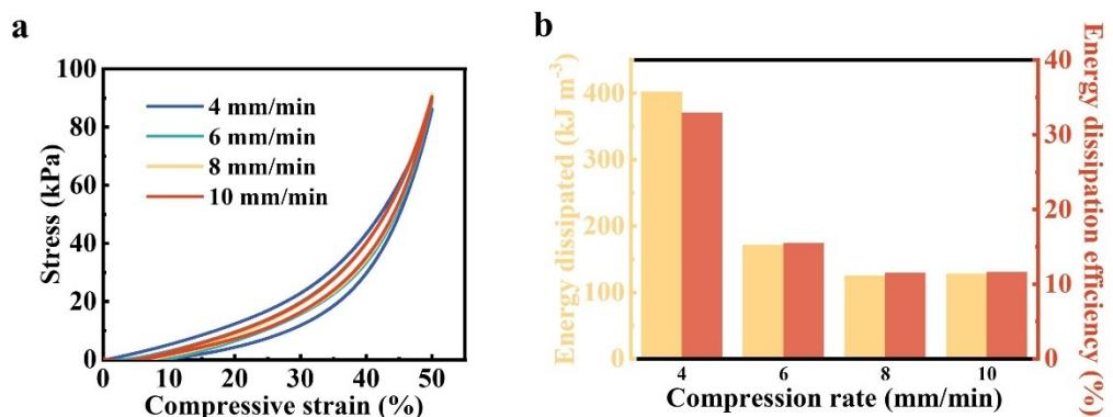
**Fig. S3:** (a) Loading-unloading test of CS<sub>1</sub>AA<sub>15</sub>AC<sub>75</sub> hydrogel at different compression rates (b) Calculation of energy dissipated at different compression rates of CS<sub>1</sub>AA<sub>15</sub>AC<sub>75</sub> hydrogel at 50% strain vs. energy dissipation efficiency.
