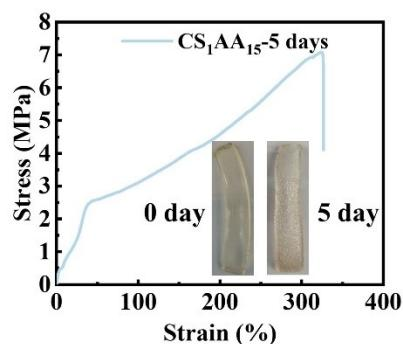
**Fig. S6:** Stress-strain curves of CS<sub>1</sub>AA<sub>15</sub> hydrogel stored at 25 °C and 54% RH for 5 days.
