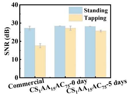
**Fig. S10:** SNR of commercial 3M electrode and electrode added CS<sub>1</sub>AA<sub>15</sub>AC<sub>75</sub> hydrogel with different storage times for detecting ECG signals
