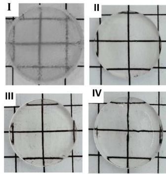
**Fig. S4:** Optical photograph of (I) CS<sub>1</sub>AA<sub>15</sub> (II) CS<sub>1</sub>AA<sub>15</sub>AC<sub>25</sub> (III) CS<sub>1</sub>AA<sub>15</sub>AC<sub>50</sub> (IV) CS<sub>1</sub>AA<sub>15</sub>AC<sub>75</sub> hydrogel transparency.
