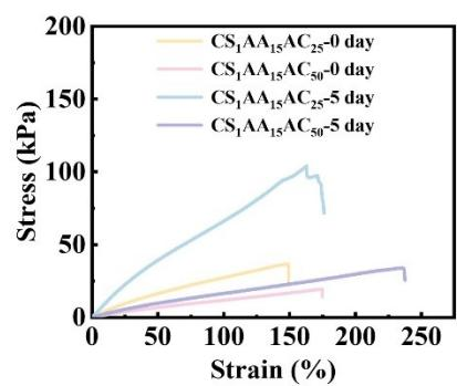
**Fig. S8:** Stress-strain curves of  $\text{CS}_1\text{AA}_{15}\text{AC}_{25}$ ,  $\text{CS}_1\text{AA}_{15}\text{AC}_{50}$  hydrogels initial and stored at 25 °C and 54% RH for 5 days
