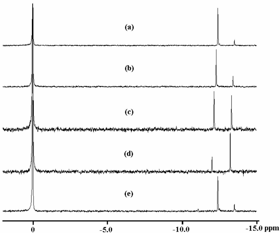
**Fig. S1** Temperature-dependent  $^{31}\text{P}$  NMR of **1** in  $\text{D}_2\text{O}$ : (a) at 23.7 °C, (b) at 39.7 °C, (c) at 58.9 °C, (d) at 79.7 °C, and (e) the solution of (d) remeasured at 24.7 °C.
