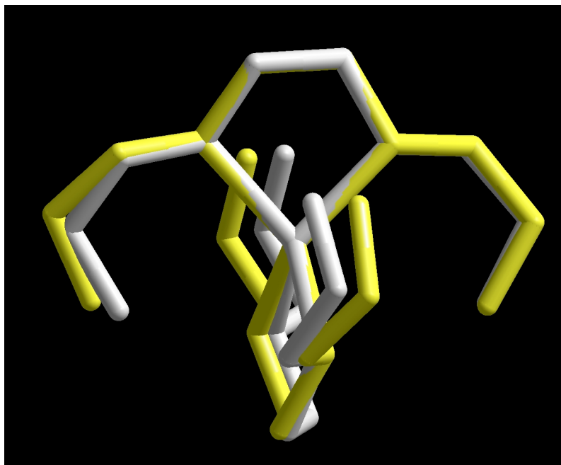
Figure S8. The crystal structure (white) and the DFT structure (yellow) of [\text{Zn}(\text{BHEEN})_2]^{2+} overlaid at the 5-membered chelate ring in the plane of the picture.
