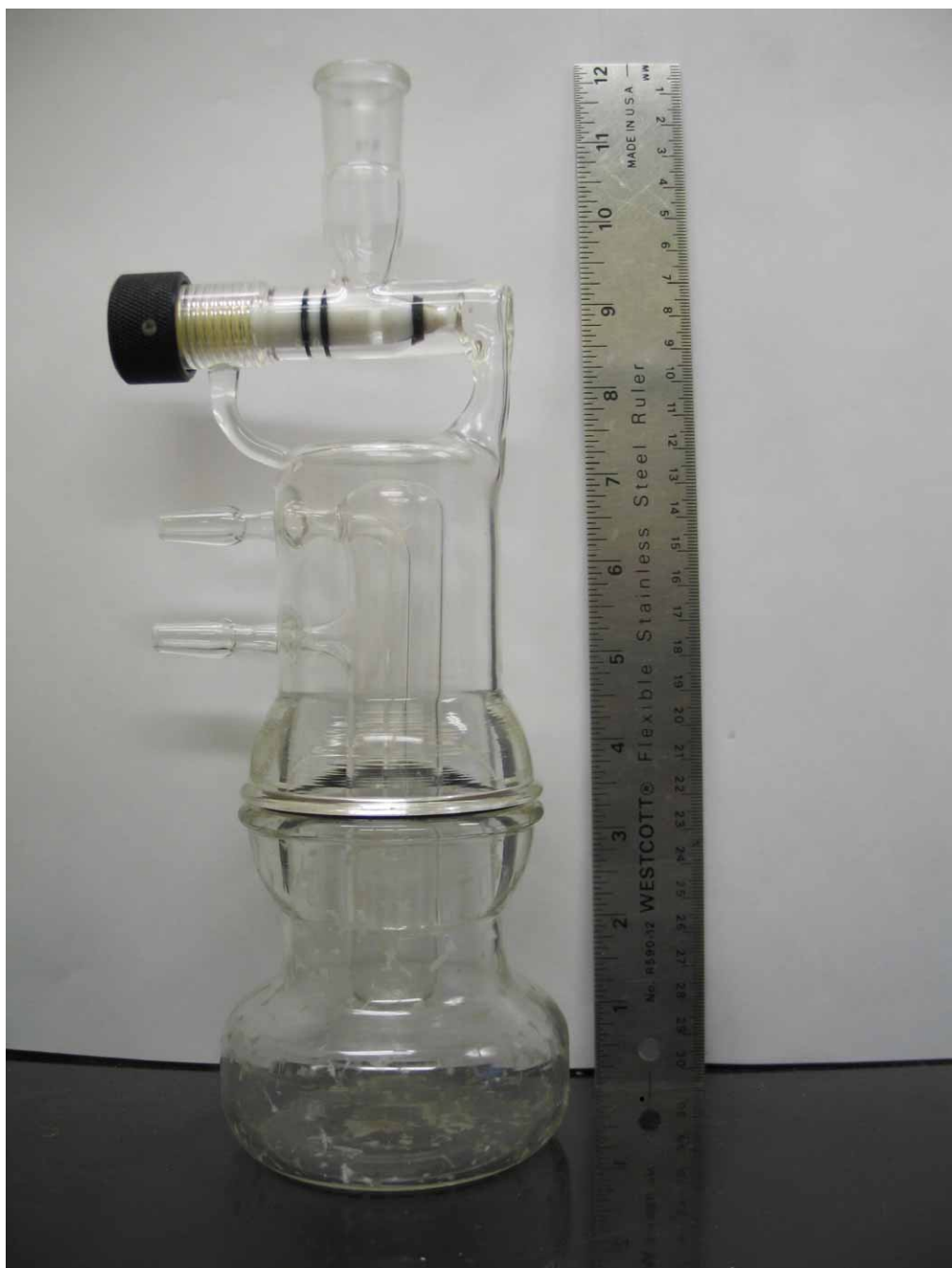
Figure S3. Sublimation vessel (Ace Glass Inc.) used for subliming Li[Al(OR F ) 4 ].
