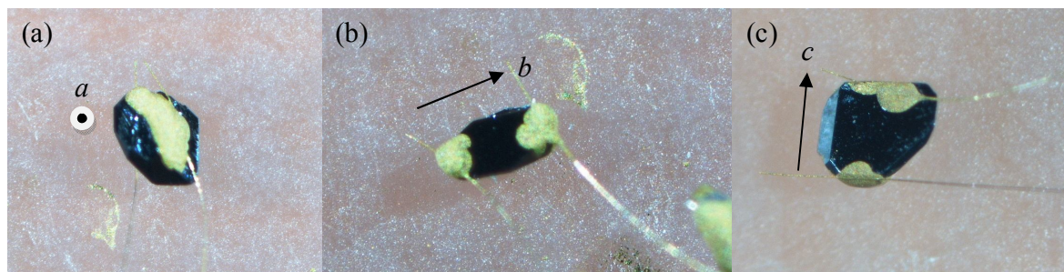
Figure S8. Single crystal for dielectric anisotropy measurements of salt 1 . Au wires were attached along the a) a -, b) b -, and c) c -axis.
