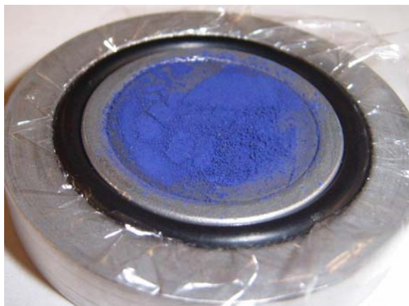
Fig. S15 PXR measurement setup for the activated PCN-82
