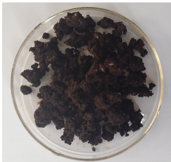
Fig. S1 A photograph of a Petri dish containing 40 g of MnFe 2 O 4 nanocrystals.
