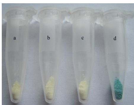
Fig. S9 Photographs of crystals of 1 soaked in DMF solution containing M(\text{NO}_3)_2 with 10^{-1} M, a) \text{Mn}^{2+} , b) \text{Co}^{2+} , c) \text{Ni}^{2+} , d) \text{Cu}^{2+} for 24 h, indicating selective color changes for \text{Cu}^{2+} .
