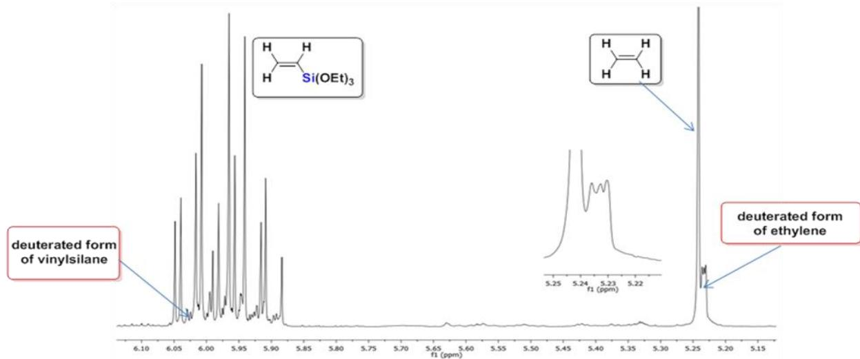
$^1\text{H}$  NMR spectrum of ethylene and deuterated ethylene as well as vinylsilane and deuterated vinylsilane observed in the reaction between (*E*)-1,2-bis(triethoxysilyl)ethene and diethylamine-*d*.
