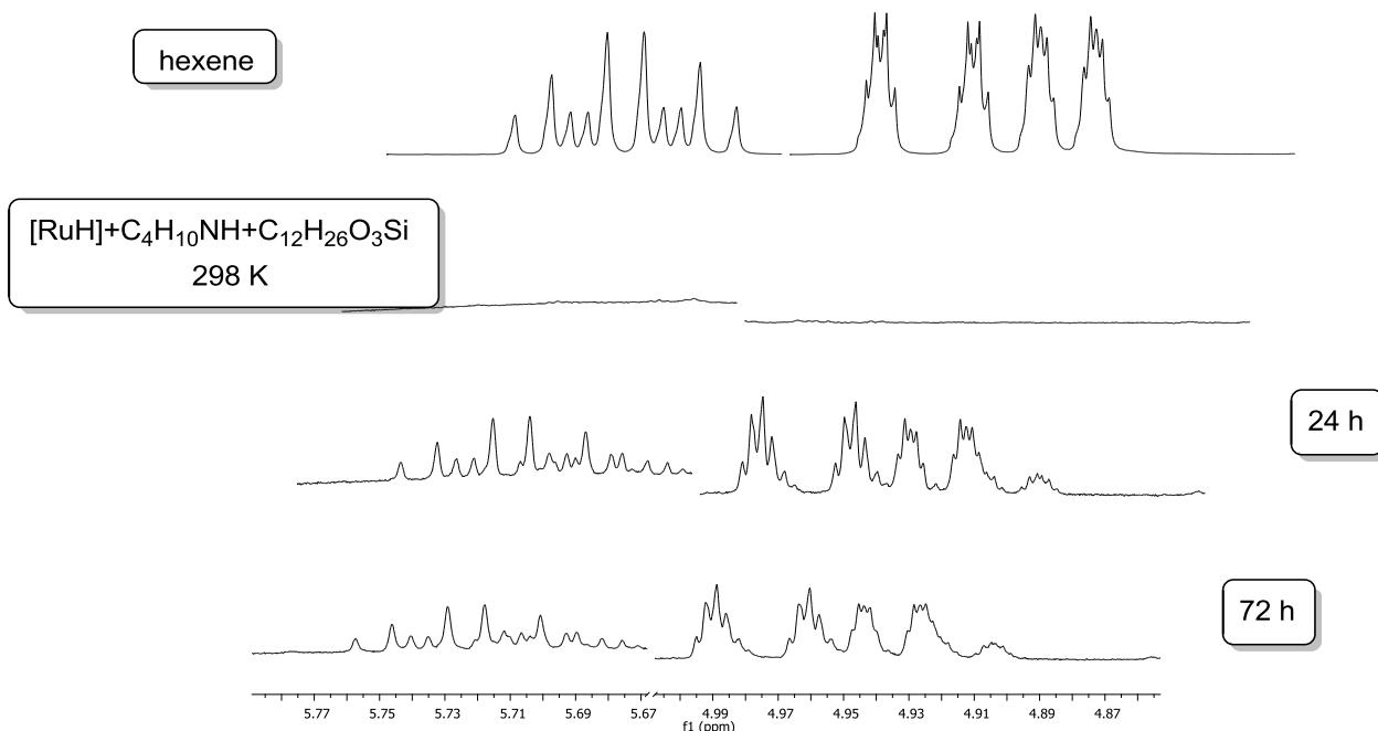
$^1\text{H}$  NMR spectra of pure hexene and hexene observed in the reaction between (*E*)-hexenyl(triethoxy)silane and diethylamine-*d*. This is evidence on the formation of olefin molecule.
