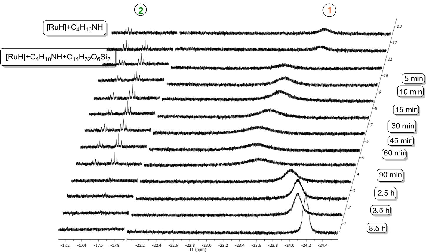
$^1\text{H}$ NMR spectra of the reaction between (*E*)-1,2-bis(triethoxysilyl)ethene and diethylamine confirming the regeneration of ruthenium-hydride **1** and the formation of two new ruthenium-hydride complexes with coordinated amine.
