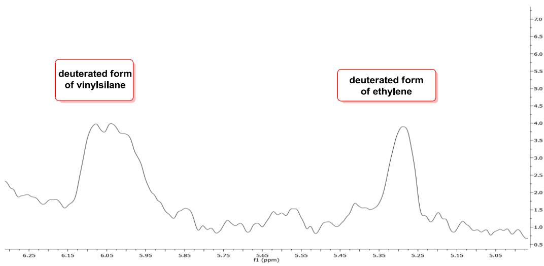
$^2\text{H}$  NMR spectrum of deuterated ethylene and deuterated vinylsilane observed in the reaction between (*E*)-1,2-bis(triethoxysilyl)ethene and diethylamine-*d* (1D sequence without decoupling using  $^2\text{H}$  lockswitch unit).
