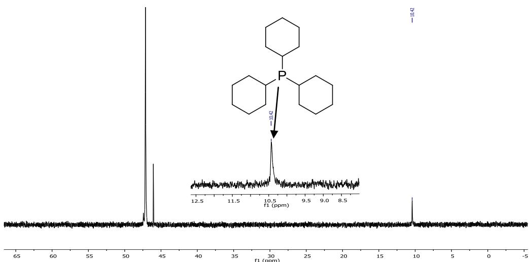
$^{31}\text{P}$  NMR spectrum confirming dissociation of free  $\text{PCy}_3$  from complex 2 after addition of bis(silyl)ethene and heating at  $120^\circ\text{C}$ .
