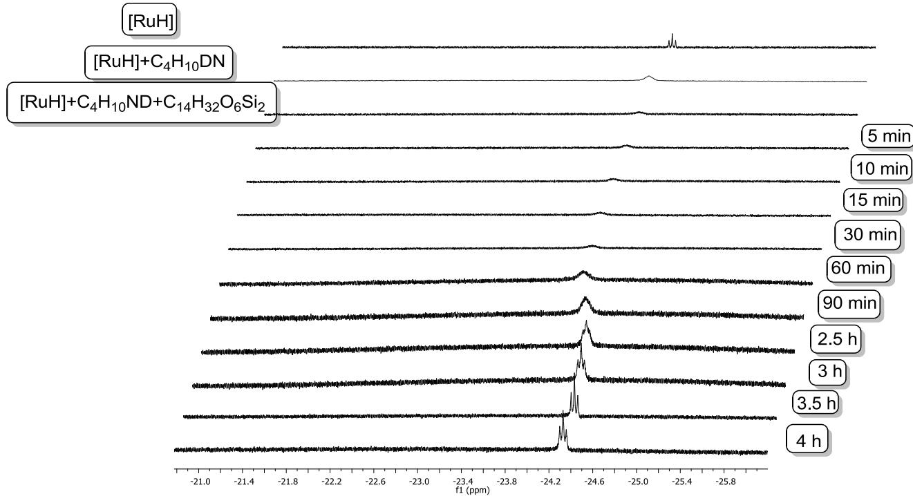
$^1\text{H}$  NMR spectra of reaction between (*E*)-1,2-bis(triethoxysilyl)ethene and diethylamine-*d* in the presence of 10 mol% of **1** confirming the regeneration of ruthenium-hydride complex **1**.
