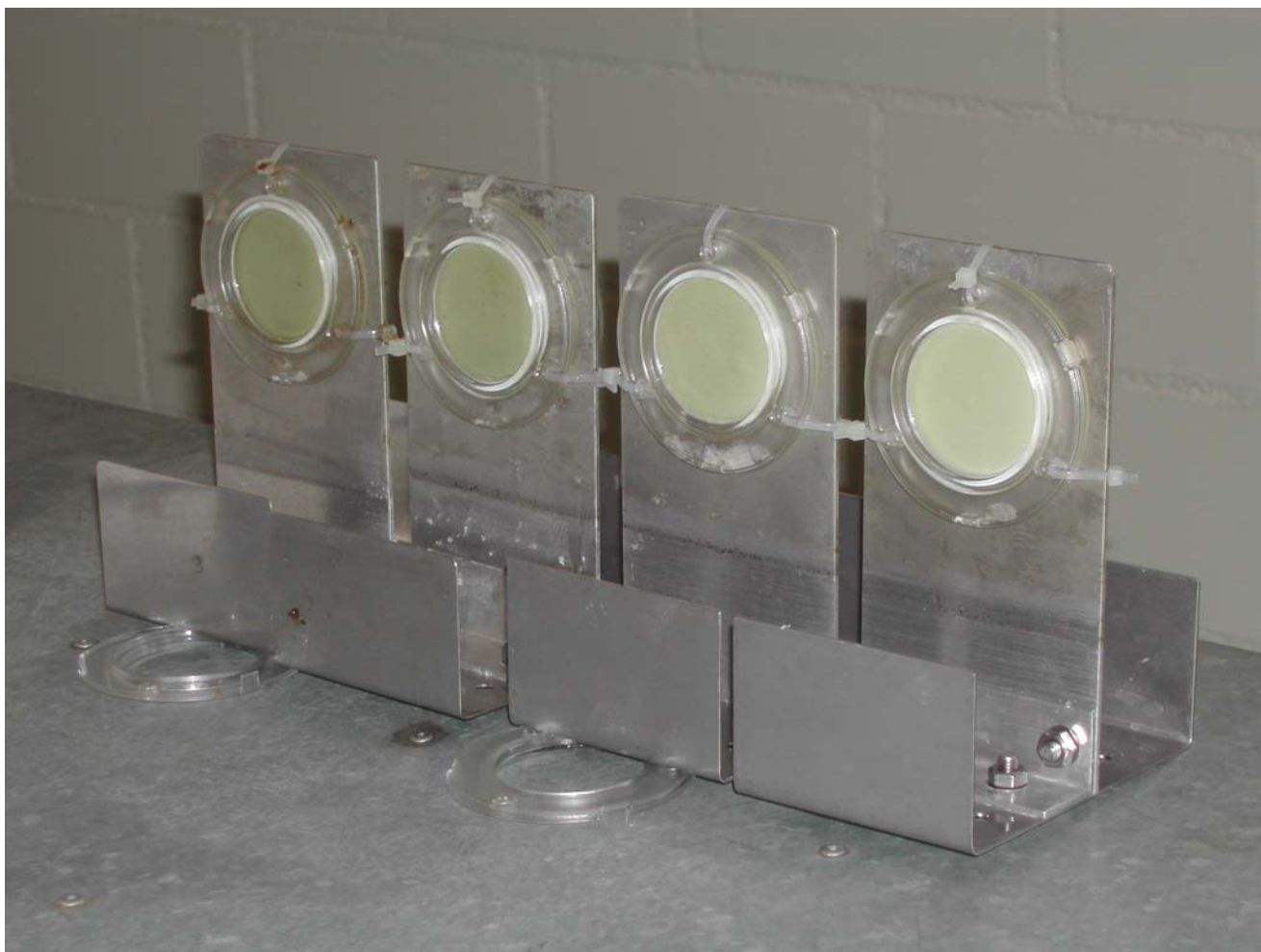
Photo 5 shows a set of SDB disks that had been exposed to treated sewage effluent for five days (note the absence of biofouling).
