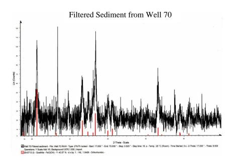
Supplementary Figure 1: XRD scan of solids obtained from Wells 2-26A (Top) and 70 (bottom). The material from Well 2-26A is a mixtures of aragonite (CaCO<sub>3</sub>) and goethite (FeO(OH)) while Well 70 contains primarily goethite. Green lines are from the aragonite, while red lines are for the goethite.
