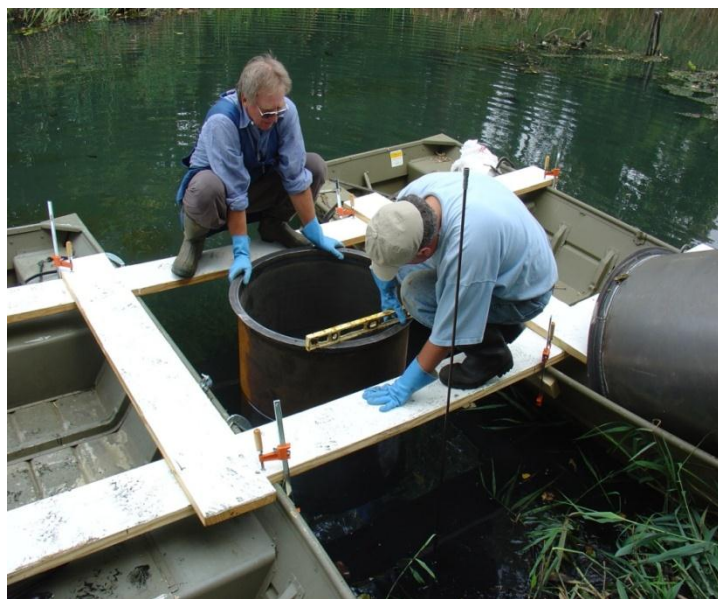
Figure S2. (a) The test cell cylinders, (b) leveling a test cell prior to attaching a collar, and (c), a long (4 ft) collar attached (with bungee cords) to the underwater test cell cylinder. The hooks on the bungee cords go through holes in the test cell cylinder and collar, keeping them aligned during installation. The collar was removed by simply removing the cords.
