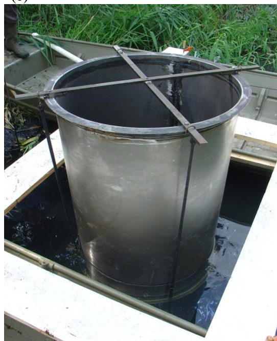
Figure S2. (a) The test cell cylinders, (b) leveling a test cell prior to attaching a collar, and (c), a long (4 ft) collar attached (with bungee cords) to the underwater test cell cylinder. The hooks on the bungee cords go through holes in the test cell cylinder and collar, keeping them aligned during installation. The collar was removed by simply removing the cords.
