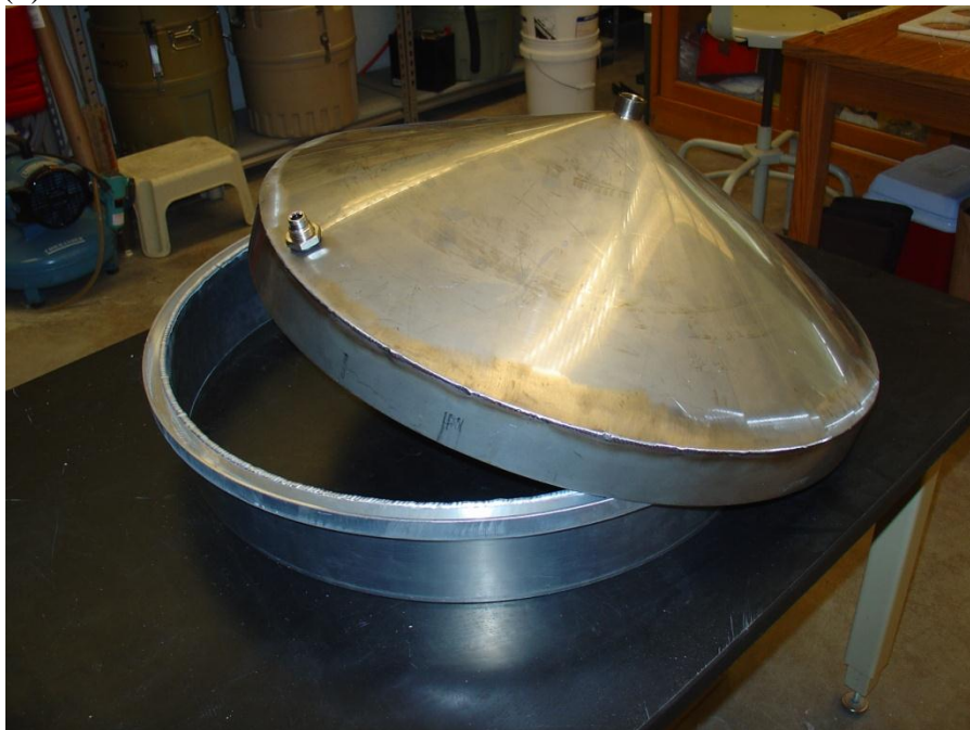
Figure S4. (a) The seepage meter flow tube, and (b) flanged cone. A water-tight seal between the two dome pieces is made by placing closed-cell foam in the u-shaped channel of the bottom (flange) piece where the rim of the top (cone) piece fits, pressing them together by attaching bungee cords.
