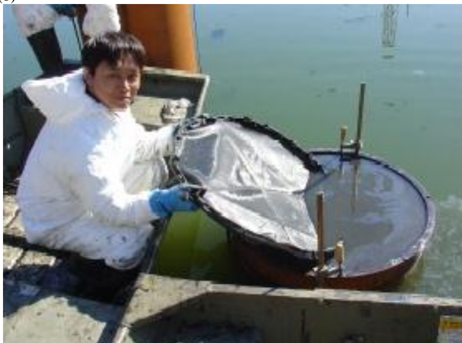
Figure S3. (a) The spring steel ring with geofabric attached, and (b) placing it in a cell after excavation. Notice the sheen of oil on top of the water in the collar. In this case, 3 ft long clamps were used to hold a 2 ft long collar to the test cell during excavation and sand addition
