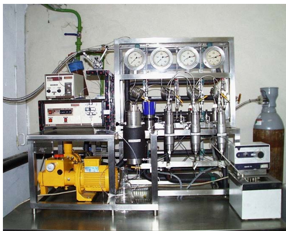
Figure S2 : picture of the SEPREX SF200 pilot used for scCO 2 extractions
