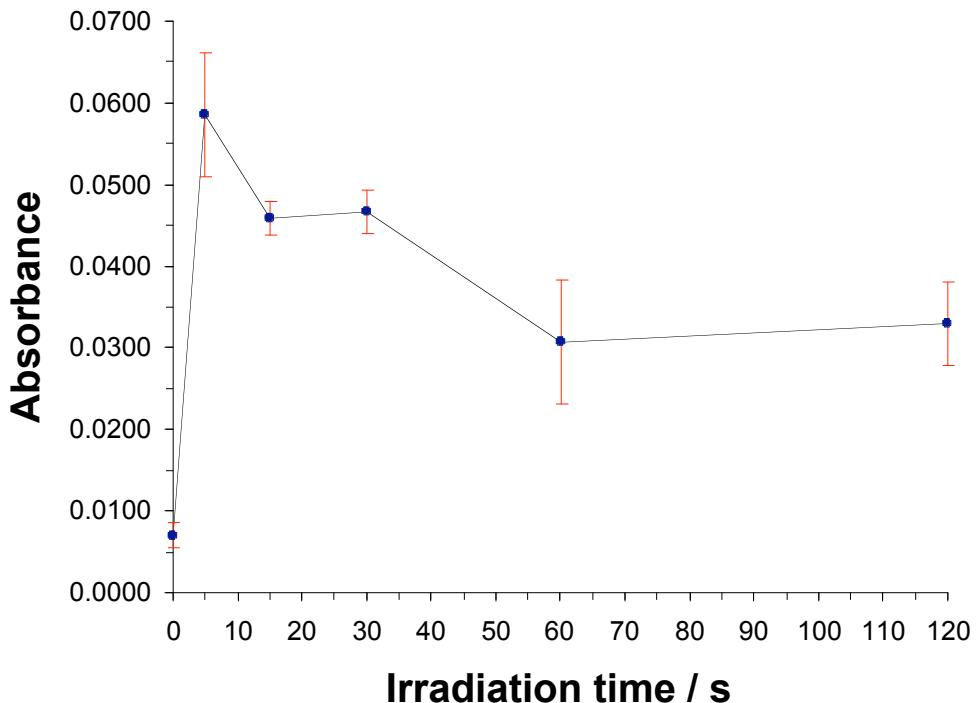
**Fig. S3. Effect of the ultrasound irradiation time on the Hg absorbance.**
