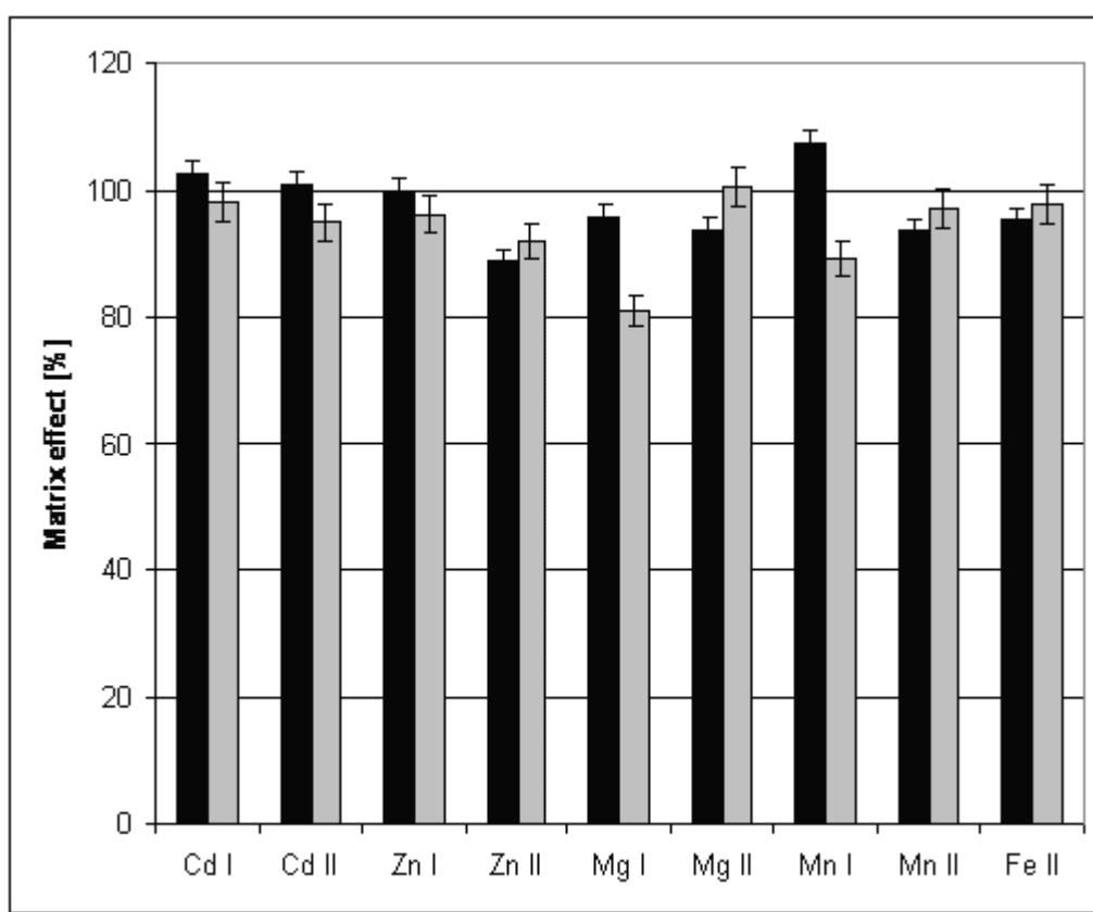
Fig. 5. The matrix effect from nitric acid on emission intensity of some metals by the Integra XL ICP-OES system with solution nebulization using NAR-1 and CCN
