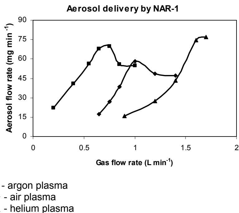
Fig. 2. The effect of nebulizer gas flow rate for argon, air and helium on aerosol flow rate produced by NAR-1 at  $0.2 \text{ ml min}^{-1}$  water consumption rate.
