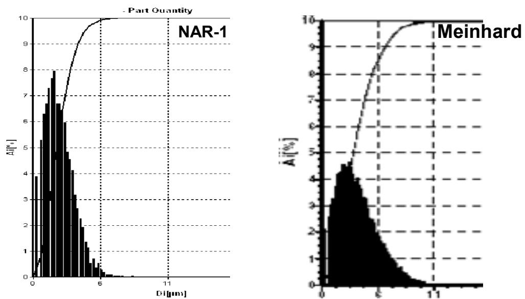
Fig. 3. The drop size distribution of tertiary aerosol obtained by NAR-1 and Meinhard nebulizers.
