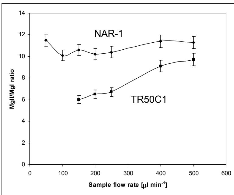
Fig. 4. The effect of sample flow rate on MgII/MgI ratio for ICP-OES systems with NAR-1 and CN (a – for Integra XL; b – for JY 138).
