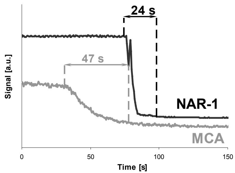
Fig. 6. The comparison of wash-out times for Zn for NAR-1 and MCA nebulizers at  $0.15 \text{ ml min}^{-1}$  of sample flow rate and  $400 \text{ ml min}^{-1}$  of nebulizer gas flow rate by MIP-OES
