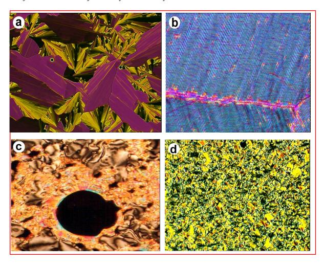
**Figure 3**: (a) The texture of  $B_1$  phase at 119.0 °C, obtained on cooling the isotropic phase of compound **1c**. On further cooling we obtain the phase  $B_x$  shown in (b). Observe the striped pattern, shown magnified (400×), formed on the fan-shaped texture of  $B_1$  phase. (c) The unspecified texture of  $B_2$  phase along with the schlieren texture in some regions) exhibited by compound **1e** at 114.5 °C and (d) schlieren texture of the B2 phase of **2e**.
