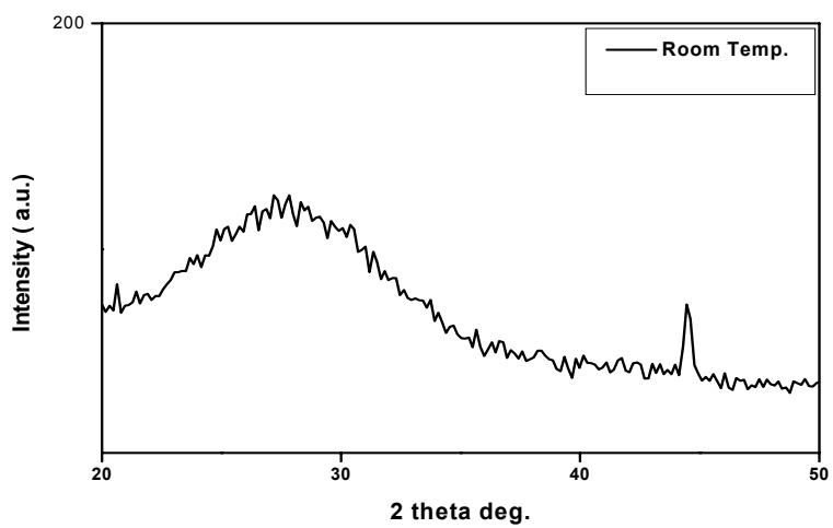
**Fig. S1** XRD of reused Q-CdS-glass powder after three times photodecompositions
