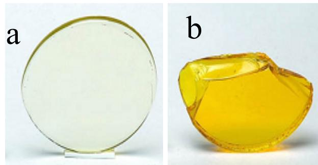
**Fig. S2** Typical photographs of glass matrix, a) before crystal growth of CdS and b) after crystal growth of CdS
