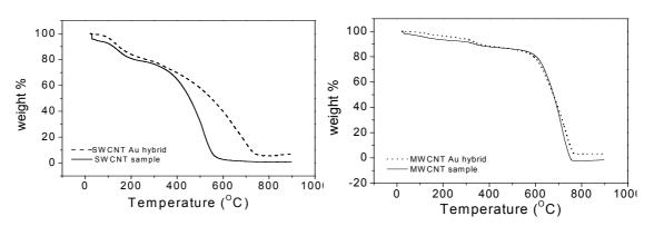
Fig. 2: TGA analysis of SWNTs and MWNTs and their gold composites.
