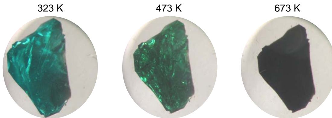
Fig. SI2 Stereomicroscopic images of Ni-Al hydrotalcite with \tau = 1 s upon in situ heating in air at different temperatures.
