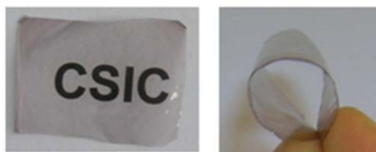
Figure S5. Flexible and transparent film of PVAPery/G
