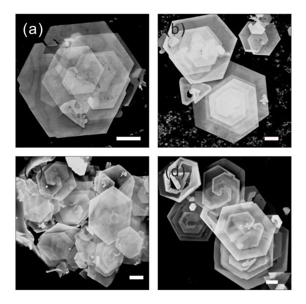
**Figure S1.** Scanning electron microscopy (SEM) images of gold spirangles synthesized from a mixture of 1 mL of Brij 700 aqueous solution (5 wt%), 0.1 mL of 10 mM NaOH (aq), and 0.1 mL of 10 mM HAuCl<sub>4</sub> (aq) after 6 h heating at 50 °C Scale bars represent: 1  $\mu$ m in (a), (b), and (d), and 2  $\mu$ m in (c).
