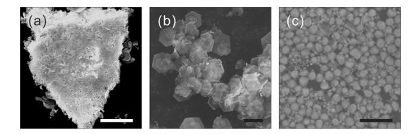
Figure S2. Scanning electron microscopy (SEM) Images of gold crystals synthesized after 6 h heating at 50 °C from a mixture of 0.1 mL of 10 mM HAuCl<sub>4</sub> (aq), 0.1 mL of 10 mM NaOH (aq), and 1 mL of (a) 2 wt%; (b) 5 wt%; (c) 10 wt% Brij 700 aqueous solution. Scale bars represent: 10  $\mu$ m in (a), 5  $\mu$ m in (b), and 1  $\mu$ m in (c).
