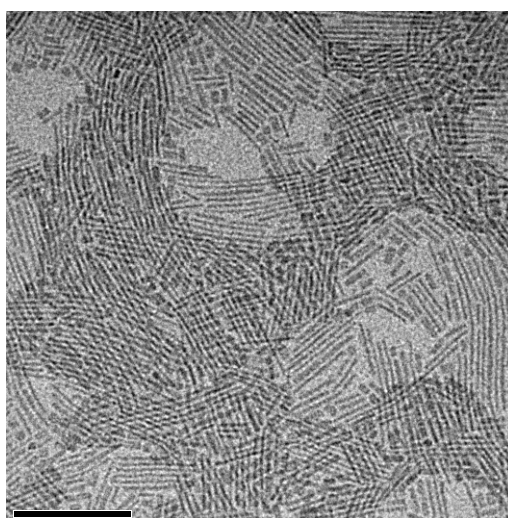
Figure S5. TEM micrograph of pure (un-doped) SrF 2 NCs prepared by thermolysis route using 80 mol% Sr(CF 3 COO) 2 as reaction precursor.
