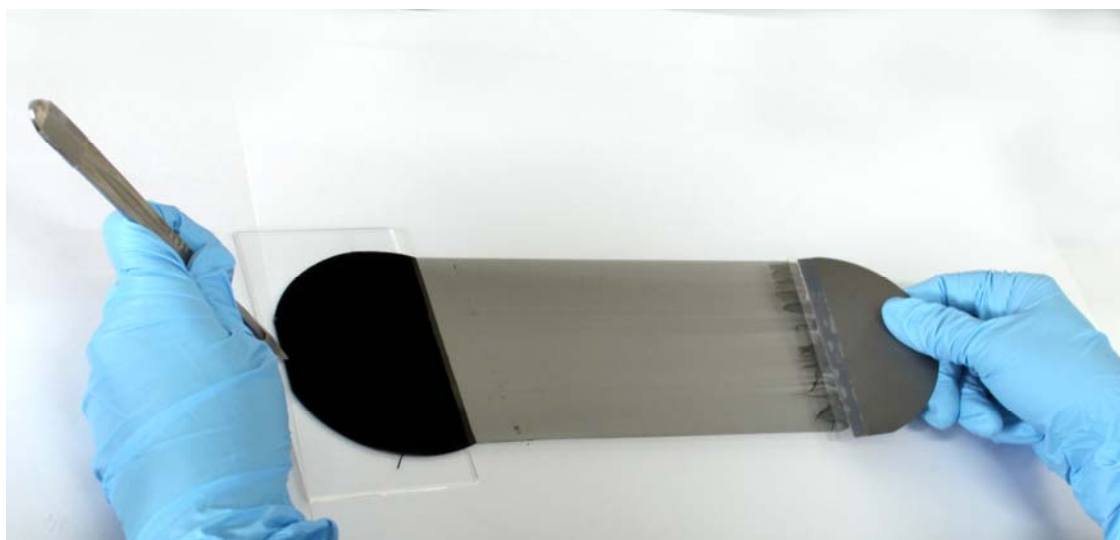
Figure S2: Photograph of a drawn film of MWCNT webs from an MWCT forest grown on a ceramic substrate.
