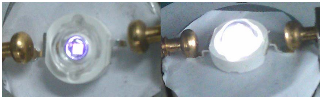
Figure S5. Photographs of a 368 nm UV LED chip (left) and the chip coated with \text{K Sr}_4(\text{BO}_3)_3:0.015\text{Dy}^{3+}, 0.005\text{Tm}^{3+}, 0.02\text{Eu}^{3+} (right).
