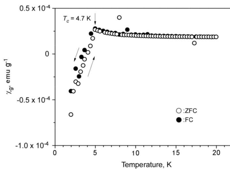
**Fig. S1.** Magnetic susceptibility of octylamine intercalated TiNCl as a function of temperature. A weak superconducting transition observed at 4.7 K is due to TiN contamination as impurity in the starting material.
