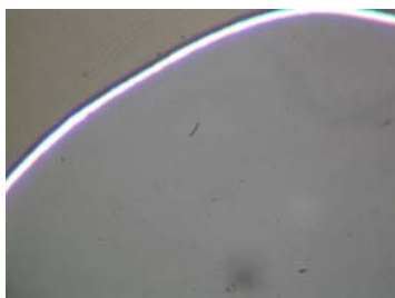
Figure 5S. Microphotograph of the SmA phase of 2 on heating (600 \times , 225 ^{\circ} C).
