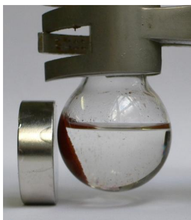
Figure S10. Application of a magnet to a diethyl ether suspension of 9 coated with \text{bmimBF}_4 (1:1 w/w).
