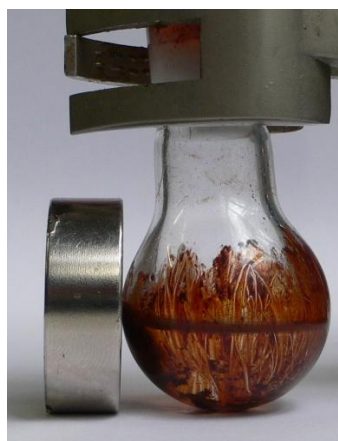
Figure S11. Application of a magnet to a diethyl ether suspension of \text{Fe}_2\text{O}_3 coated with \text{bmimBF}_4 (1:1 w/w).
