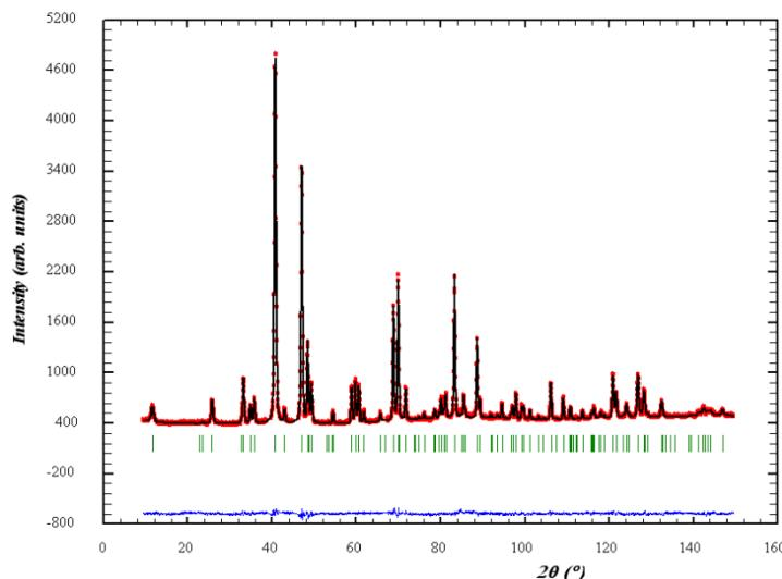
Results of Rietveld analysis against neutron powder diffraction data collected at 1173 K in air on  $\text{NdBaCo}_2\text{O}_{5+x}$  sample. The red circle symbols and the black line correspond to the observed and calculated intensities, respectively. Short vertical bars indicate the position of Bragg reflections within the  $P4/mmm$  space group (N°123). The difference between the observed and calculated profiles is plotted at the bottom. The wavelength of the incident neutrons beam is 1.594 Å.
