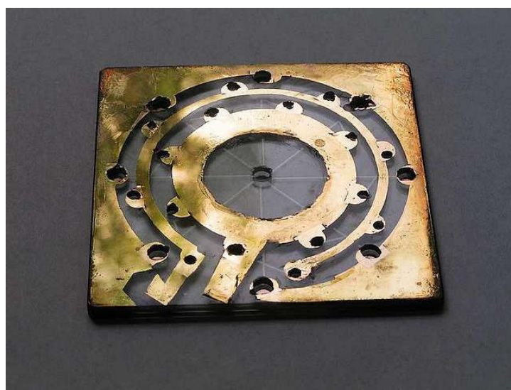
Fig. S1 Photograph of the multilayer microchip.
