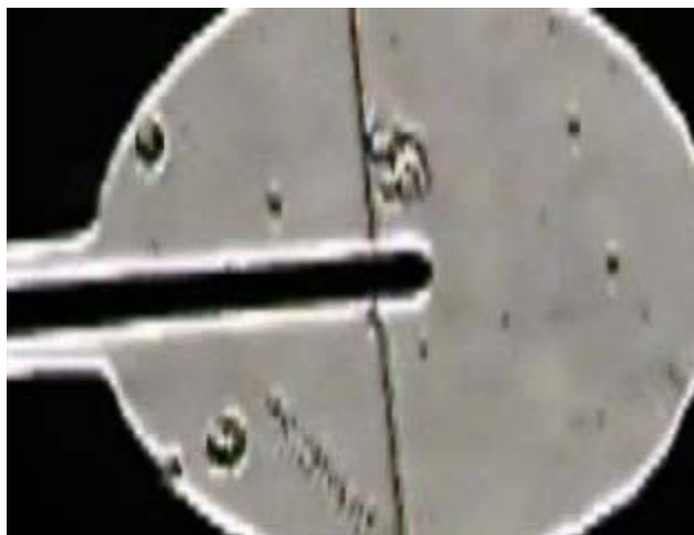
Movie S1. Attraction of cells to the edge of the sensing electrode by positive dielectrophoresis. The full movie lasts 11 seconds. Here the snapshot was taken just before the cell was trapped at the edge of the central electrode (region of strongest electric field). 5V at 1MHZ were applied across the electrodes.
