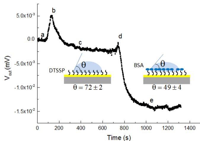
**Fig. S2** Comparisons between the signal change of the cantilever sensor chips and contact angle measurement of sessile drops.
