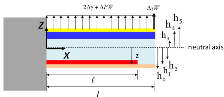
**Fig. S1** Mechanics model of a multilayer cantilever for capillary force detection
