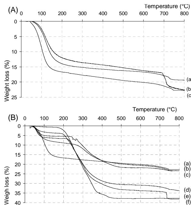
Figure SM1: thermogravimetric curves of surfactant-free materials (1) : (a) RL ; (b) 473 K – DL ; (c) SDL and Brij58/laponites materials (2): (a) SDL, (b)SDL/B-2, (c) SDL/B-4, (d) SDL/B-6, (e) SDL/B-8 and (f) physical blend of Brij58 and Quartz
