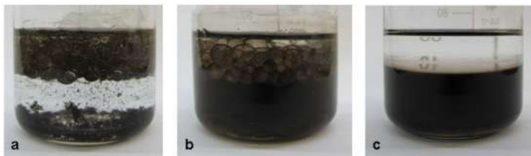
Fig. S7 Vigorous stirring without sonication, (a) pH = 1, (b) pH = 6.5, (c) pH = 12, big spheres were created at acidic and neutral pH, while almost no sphere were created at alkaline pH. This indicated that sonication had an important role in GO microsphere creation.
