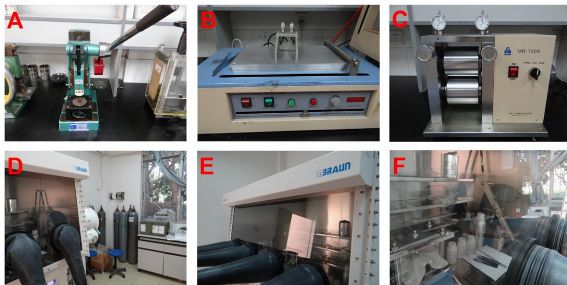
Figure S1. Main devices, materials, and battery assembly methods. (A) Agate mortar is used to triturate carbon electrode materials, an precision disc cutter is used to shape carbon electrode sheet. (B) Compact tape casting film coater with dryer is applied to coat carbon electrode materials onto carbon paper to make carbon electrode sheet. (C) Electric precision 4" width rolling press with dual micrometer is used to planish carbon electrode sheet. (D) Argon-filled glove box and argon tank. (E) Lithium tablets are stored in the glove box. (F) Lithium tablets, electrolytes, micropipette, button battery box set, battery separator, compact hydraulic crimping machine, disassembling machine, etc.
