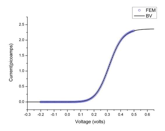
Finite Element Model predicted voltammetry response for a single potential sweep (from -0.2 V to 0.5 V) for a hemispherical electrode with radius R=25nm. The Finite Element Model(FEM) solution (blue circles) follows the behavior predicted by the Butler-Volmer equation for a one-step, one-electron process<sup>1</sup> (solid line):
