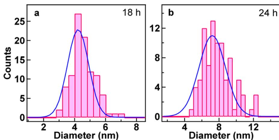
**Fig. S4** Size distributions of the Au nanoparticles decorated on the exterior surface of the sulfide nanostructures produced by the hydrothermal process for (a) 18 h and (b) 24 h, respectively. The average sizes for (a) and (b) are  $(4.2 \pm 0.7)$  and  $(7.2 \pm 1.5)$  nm, respectively.
