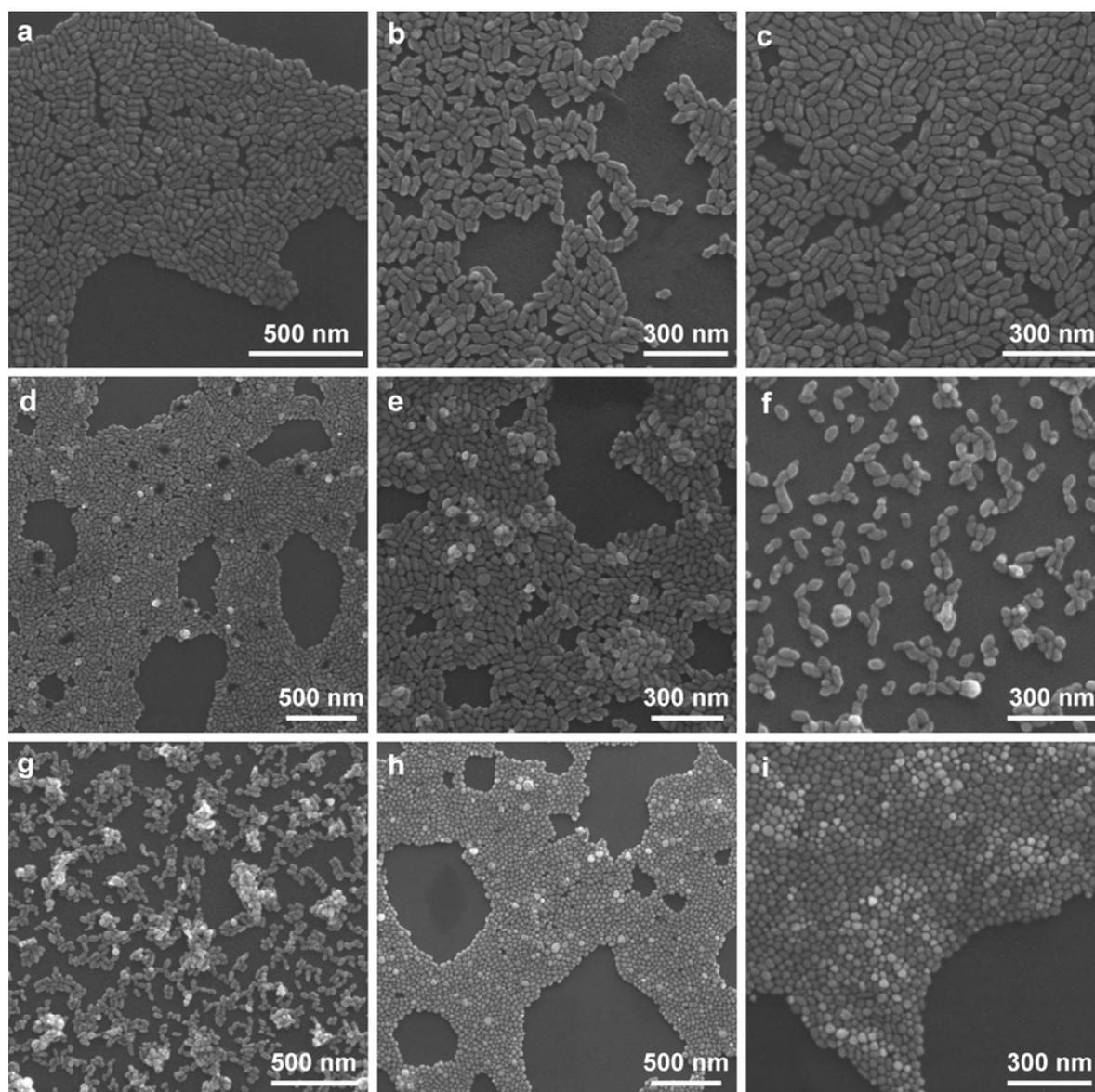
**Fig. S2** (a–i) SEM images of the hybrid gold–gold silver sulfide nanostructures obtained from the hydrothermal process for 3, 6, 9, 12, 15, 18, 24, 36, and 48 h, respectively. The SEM imaging was carried out on an FEI Quanta 400 microscope equipped with an Oxford EDX analysis system. The nanostructure samples were deposited on conductive Si substrates for the SEM imaging.
