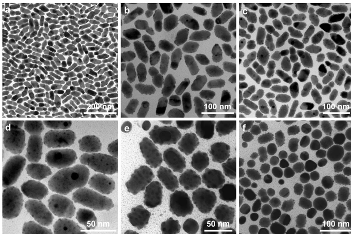
**Fig. S1** (a–f) TEM images of the hybrid gold–gold silver sulfide nanostructures obtained from the hydrothermal process for 6, 12, 15, 18, 36, and 48 h, respectively. The low-magnification imaging was performed on an FEI CM120 microscope.
