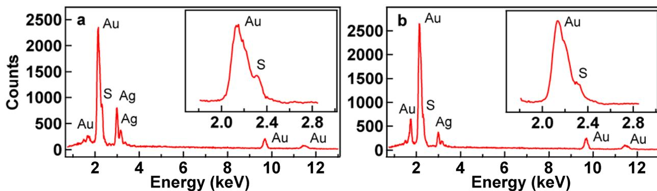
**Fig. S5** EDX spectra of the hybrid gold–gold silver sulfide nanostructures produced by the hydrothermal process for (a) 3 h and (b) 15 h.
