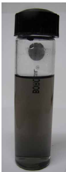
Graphene dispersion with loading 0.015 mg/ml
