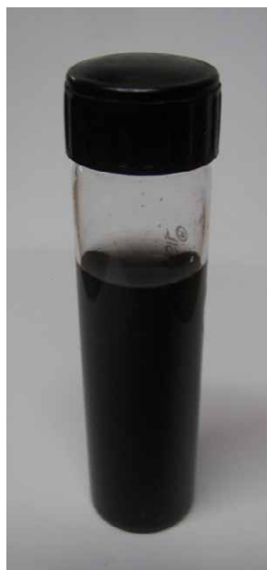
Graphene dispersion with 0.05 mg/ml loading
